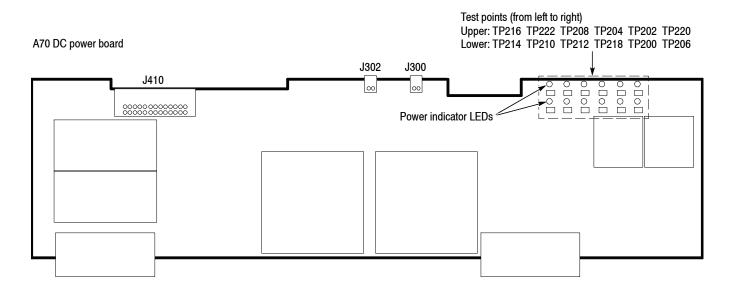
Figure 5-38: A70 DC power supply board
