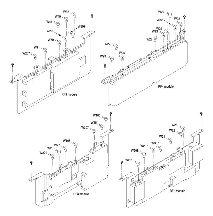
Figure 5-15: RF modules removal
