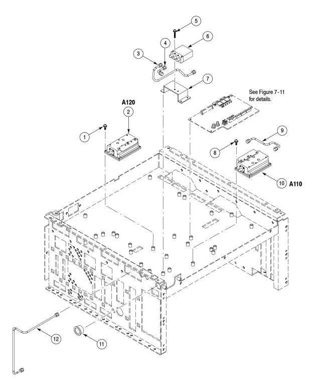
Figure 7-9: Bottom modules - RF1 (RSA3303B)
