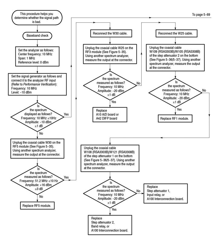
Figure 5-34: Troubleshooting procedure 3 — Signal path
