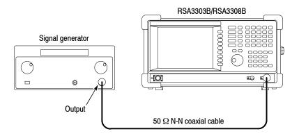
Figure 3-12: Hookup for checking the absolute amplitude accuracy
