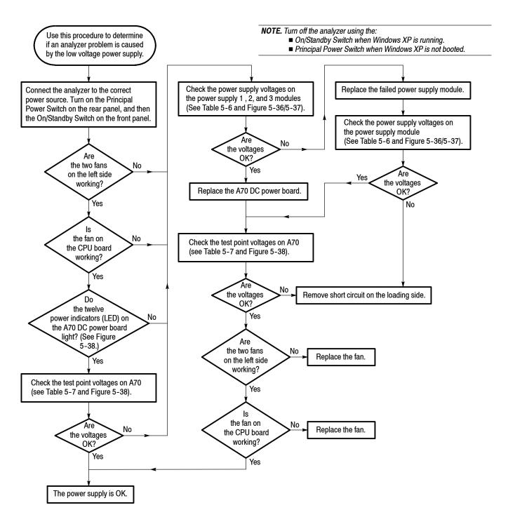
Figure 5-32: Troubleshooting procedure 1 — Power supply system
