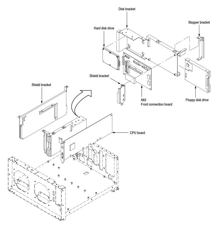
Figure 5-4: CPU board and disk modules
