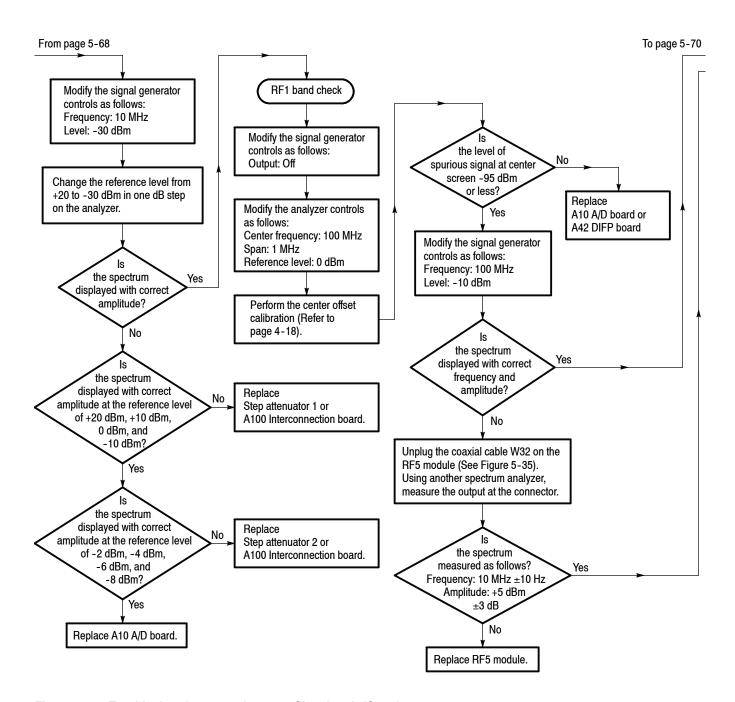
Figure 5-34: Troubleshooting procedure 3 — Signal path (Cont.)
