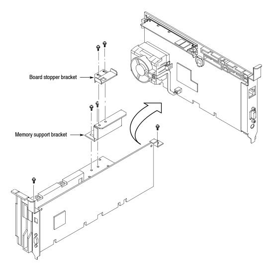
Figure 5-16: CPU board removal
