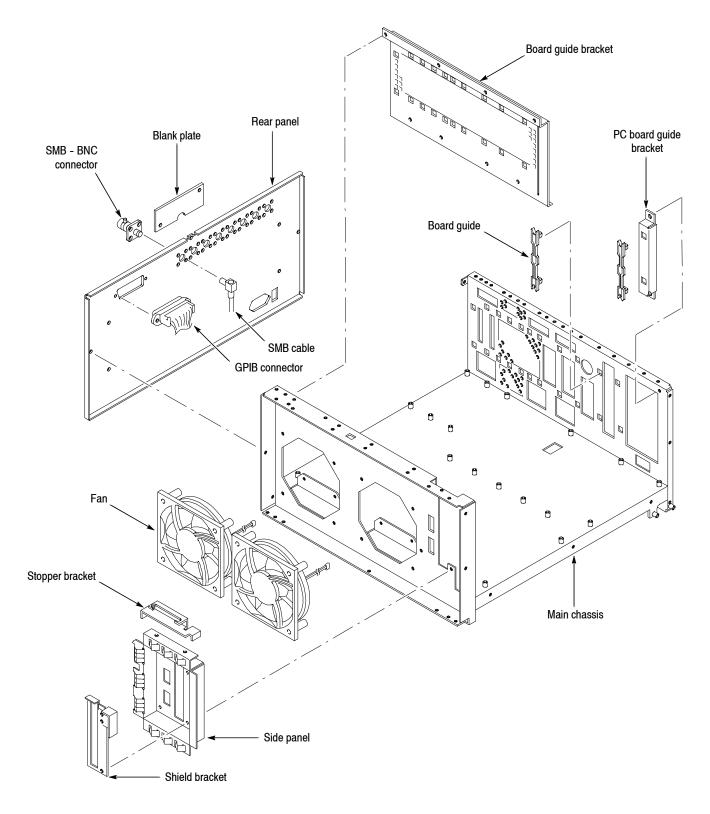
Figure 5-10: Chassis modules
