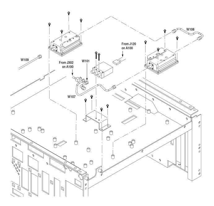
Figure 5-24: RF1 modules removal - 2 (RSA3303B)
