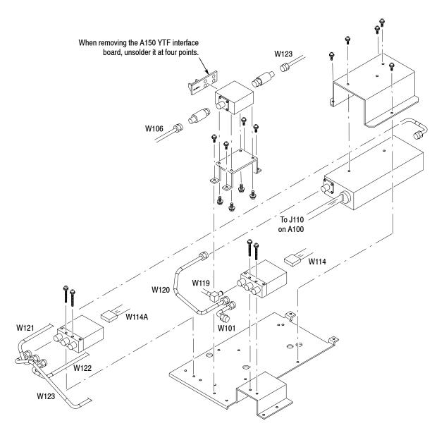
Figure 5-25: RF1 modules removal - 2 (RSA3308B)
