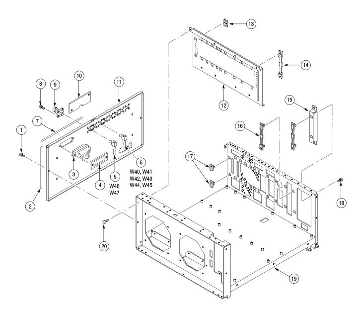
Figure 7-12: Chassis modules - 1
