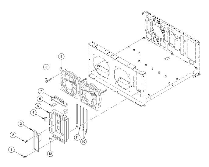
Figure 7-13: Chassis modules - 2
