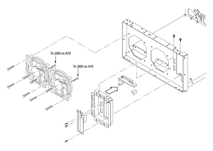
Figure 5-29: Fan and side panel removal
