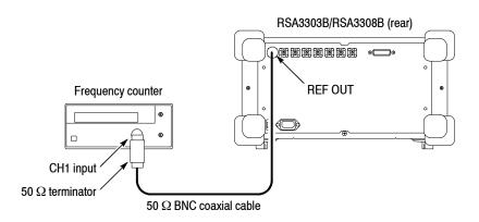
Figure 3-8: Initial test hookup
