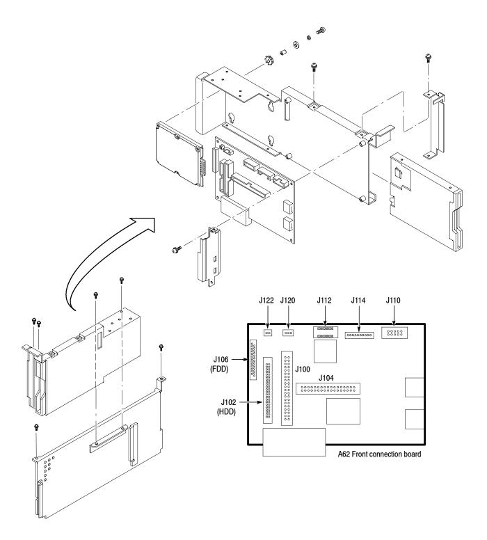
Figure 5-17: Disk module removal
