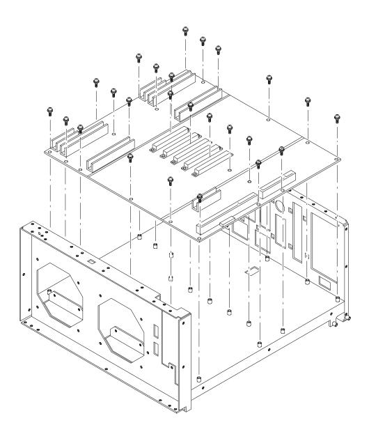
Figure 5-20: Motherboard removal
