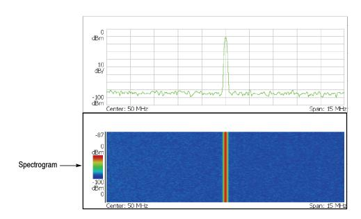
Figure 3-4: Spectrogram display
