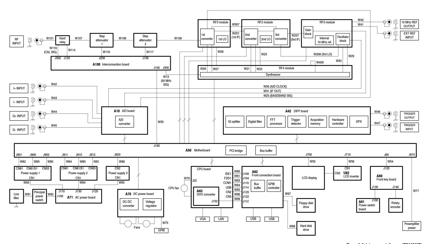
Figure 6-2: Interconnect diagram (RSA3303B)
