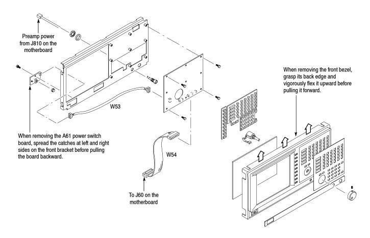
Figure 5-27: Front panel modules removal
