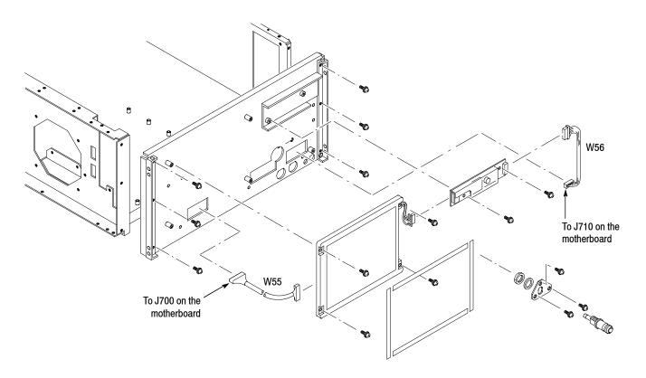
Figure 5-28: LCD display removal
