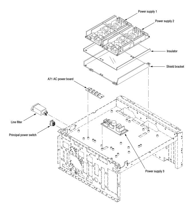
Figure 5-6: Bottom modules - Power supply
