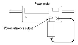
Figure 4-3: Hookup for calibrating the power sensor
