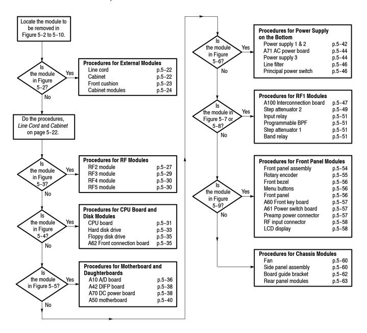
Figure 5-11: Guide to removal procedures
