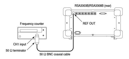
Figure 4-12: Initial test hookup
