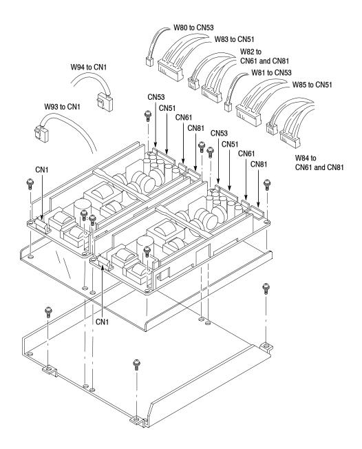
Figure 5-21: Power supply 1 and 2 removal
