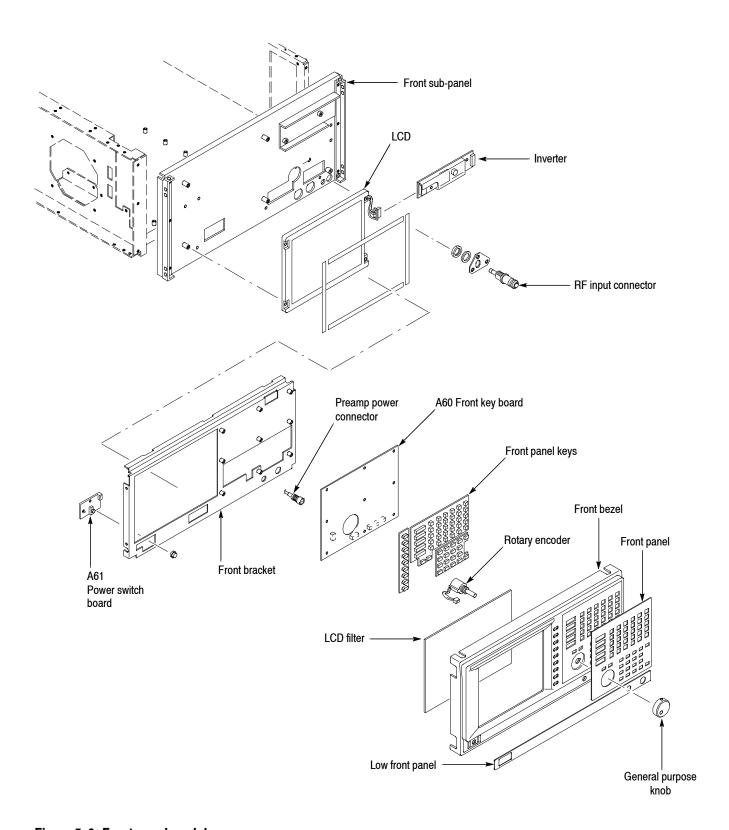
Figure 5-9: Front panel modules
