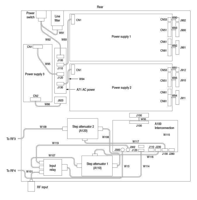
Figure 5-36: Bottom view for cable interconnection (RSA3303B)
