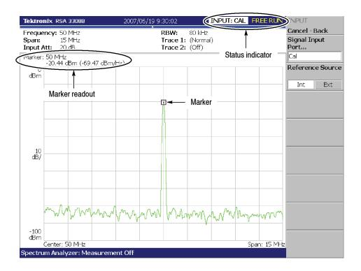
Figure 3-1: Spectrum of the calibration signal (50 MHz, -20 dBm)
