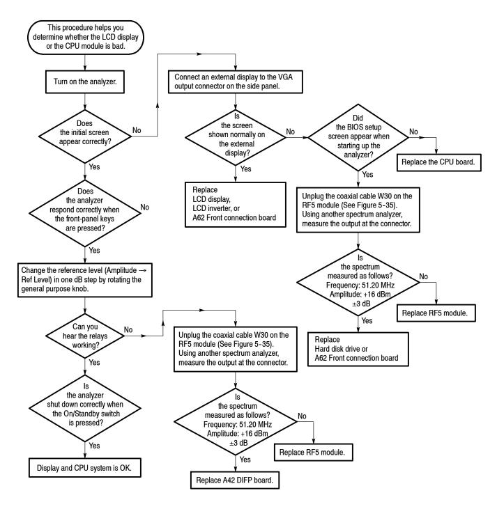
Figure 5-33: Troubleshooting procedure 2 — Display and CPU system
