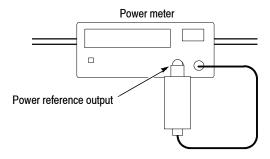
Figure 4-5: Hookup for calibrating the power sensor
