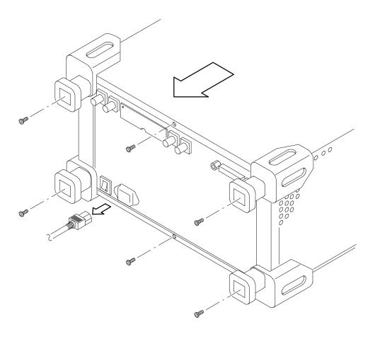
Figure 5-12: Line cord and cabinet removal
