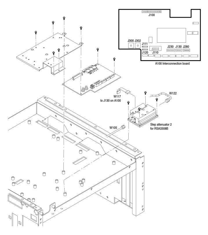
Figure 5-23: RF1 modules removal - 1
