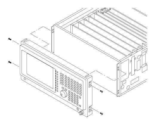
Figure 5-26: Front panel assembly removal
