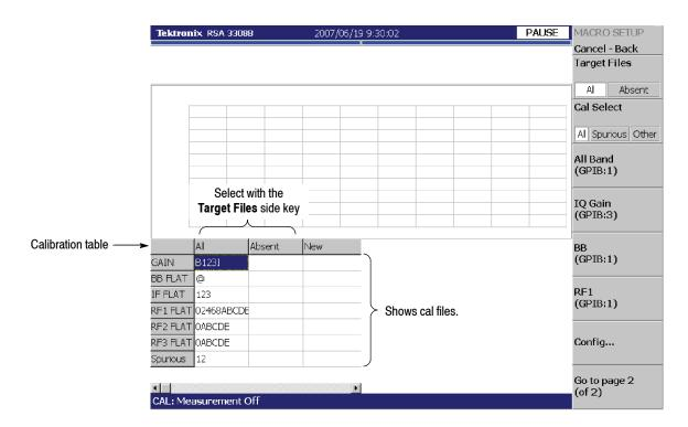
Figure 4-10: Auto calibration initial screen
