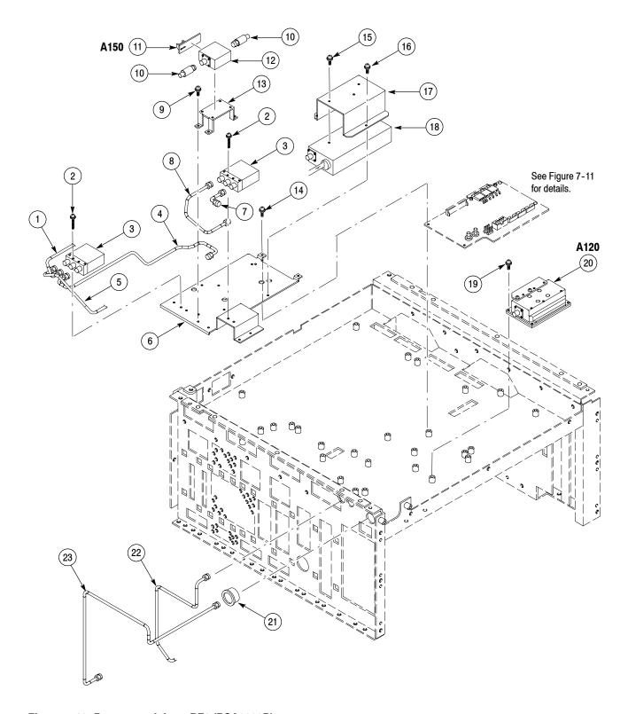
Figure 7-10: Bottom modules - RF1 (RSA3308B)
