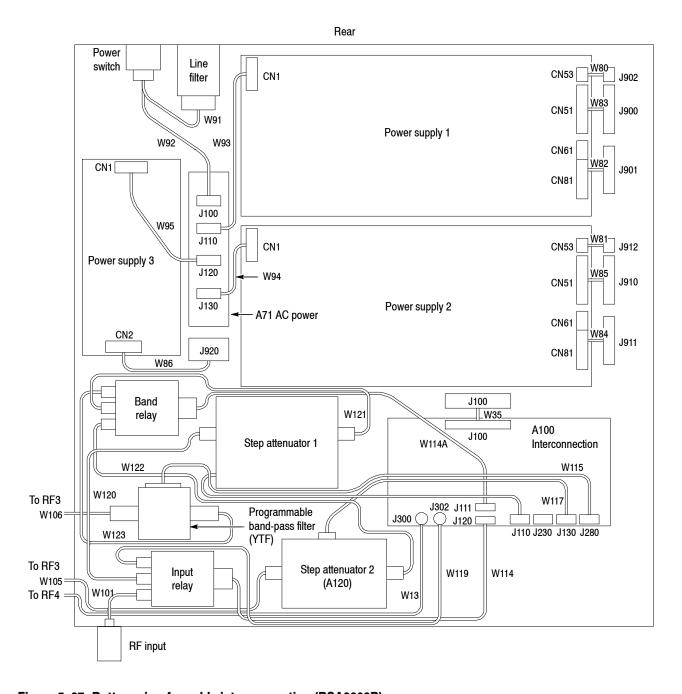
Figure 5-37: Bottom view for cable interconnection (RSA3308B)
