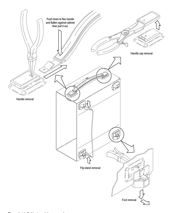
Figure 5-14: Cabinet modules removal
