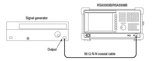
Figure 3-15: Initial test hookup
