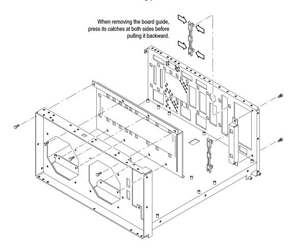
Figure 5-30: Board guide bracket removal
