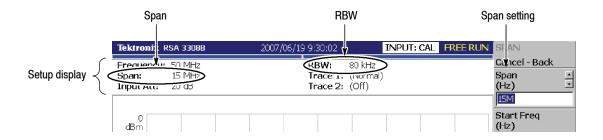
Figure 3-2: Setup display
