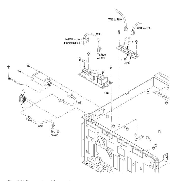
Figure 5-22: Power supply modules removal
