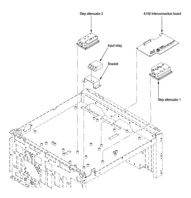
Figure 5-7: Bottom modules - RF1 (RSA3303B)
