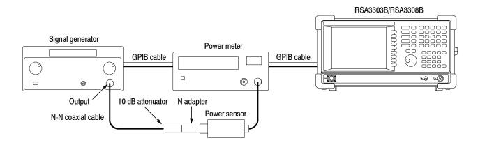
Figure 4-4: Initial test hookup
