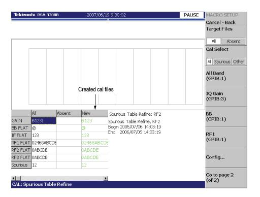
Figure 4-11: Auto cal result display example
