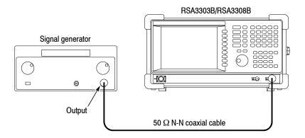
Figure 3-13: Initial test hookup
