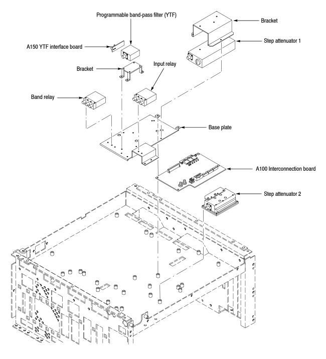
Figure 5-8: Bottom modules - RF1 (RSA3308B)
