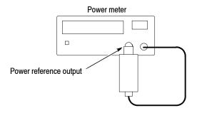
Figure 3-10: Hookup for calibrating the power sensor
