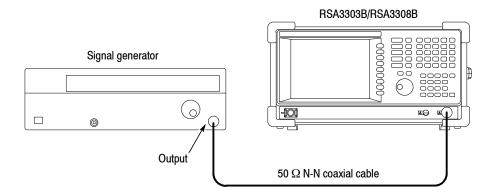
Figure 3-16: Initial test hookup
