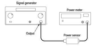
Figure 3-11: Hookup for setting the signal generator output
