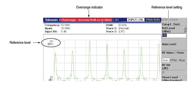
Figure 3-3: Reference level setting and overrange indicator
