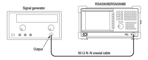
Figure 3-14: Initial test hookup
