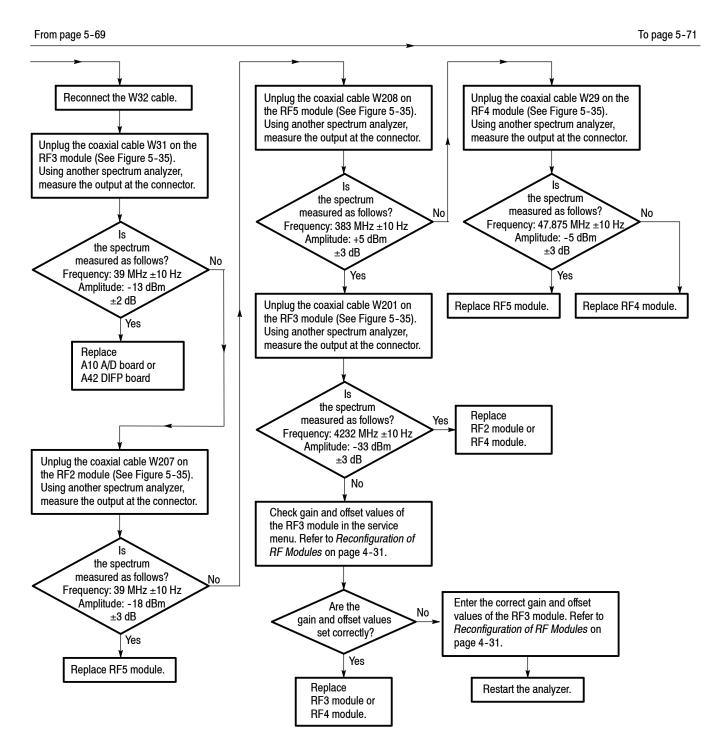
Figure 5-34: Troubleshooting procedure 3 — Signal path (Cont.)
