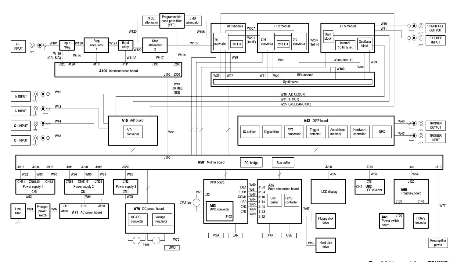
Figure 6-3: Interconnect diagram (RSA3308B)
