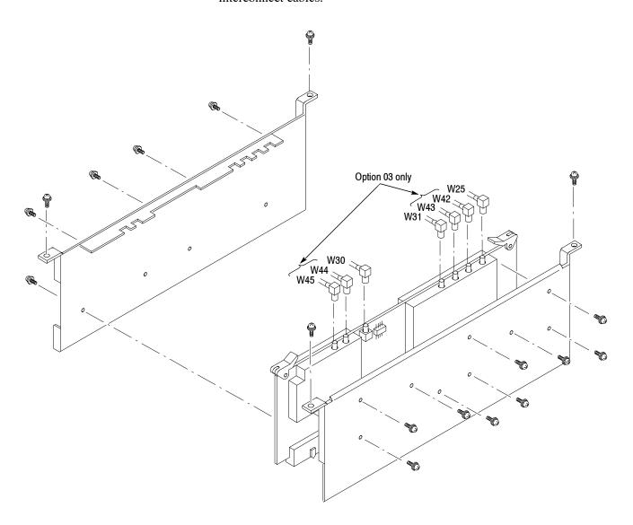
Figure 5-18: A10 A/D board removal
