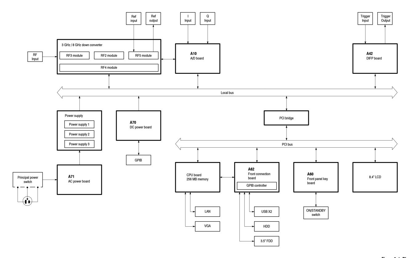
Figure 6-1: Block diagram
