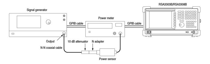
Figure 4-2: Initial test hookup
