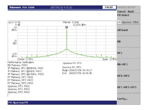
Figure 3-7: Auto test result display example
